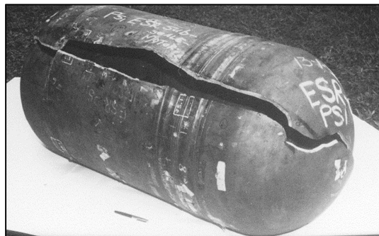
Figure 2: Failure by Excessive Plastic Deformation in Vessel Purposely Tested to Destruction
